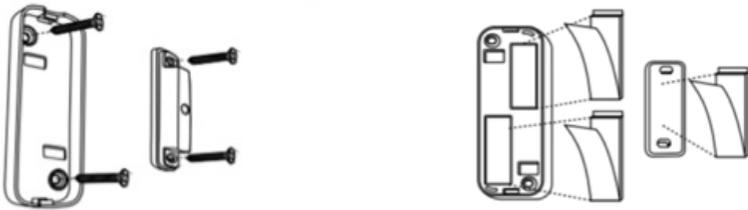
2. Once the Mount Plates are each attached to a surface, complete the installation by attaching the corresponding sensors to the plates by snapping them on.
