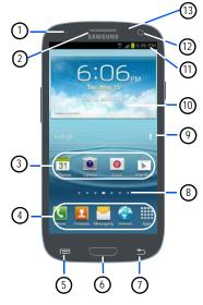
Status light: displays red when charging, green when fully charged, blue when powering up, and orange when a notification has arrived.
