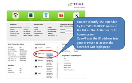
4. When you determine the IP address assigned to your WCB3000 and then enter that IP address into the address bar of your browser, you will be led to the WCB3000N graphical user interface (GUI) Login page.
