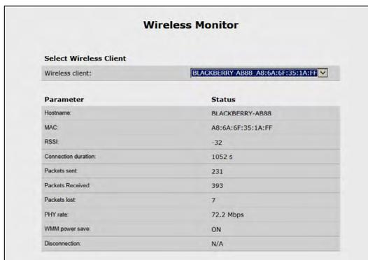
Clicking on the “Modemstatus Wireless Monitor” button at the bottom of the Wireless Status screen generates the “Wireless Monitor” screen. From here, the user can view real-time statistics specific to clients connected to the Gateway’s wireless network. To view, select a client from the “Wireless Client” drop-down list. Its statistics will appear in the lower section of the screen.
